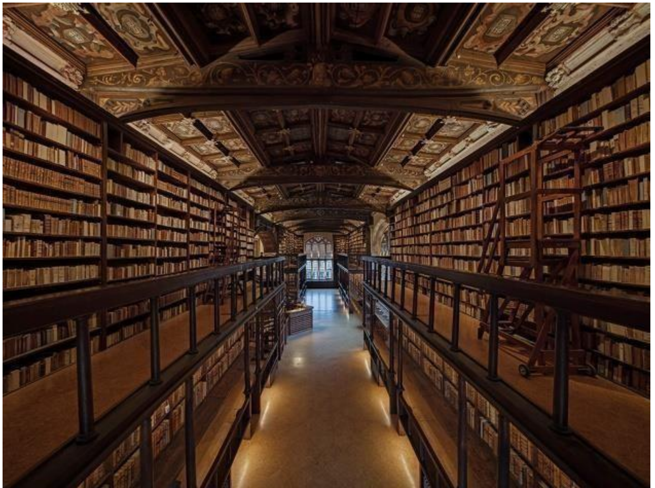
The Arts End of the library features wall wash LED luminaires for the low-level bookcases and fibre optics for the high-level bookcases. Photography: © Dan Paton www.danpaton.net
